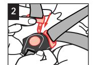
Push each buckle plate into buckle until you hear a "click". Remember to always pull up on harness straps to make sure buckle is locked tightly.
